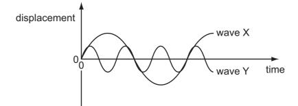
Wave X has amplitude 8 cm and frequency 100 Hz.
