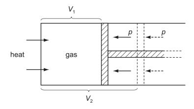
Initially, the gas has a volume  $V_1$  and is in equilibrium with an external pressure *p*. The gas is then heated slowly so that it expands, pushing the piston back until the volume of the gas has increased to  $V_2$ .
