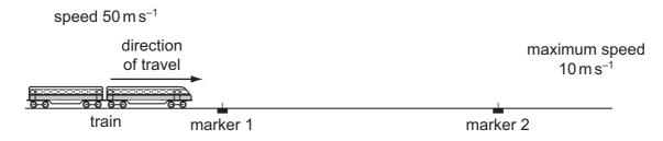
Trains coming from the left travel at a speed of  $50 \text{ m s}^{-1}$ . At marker 1, the driver must apply the brakes so that the train decelerates uniformly in order to pass marker 2 at no more than  $10 \text{ m s}^{-1}$ .
